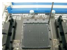
STEP 1: Lift Up The Socket Lever
