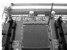
STEP 1: Lift Up The Socket Lever
