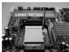
STEP 1: Lift Up The Socket Lever
