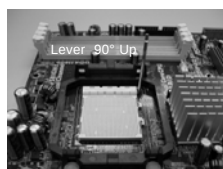
STEP 1: Lift Up The Socket Lever
