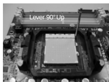
STEP 1: Lift Up The Socket Lever
