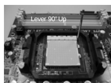
STEP 1: Lift Up The Socket Lever
