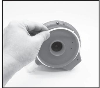
2. Use the screwdriver to unscrew the 4 screws located at the bottom of the head to release the bottom plate first. Then unscrew all the screws at the base as shown. Remove the impeller and pry open the base to expose head inside.
