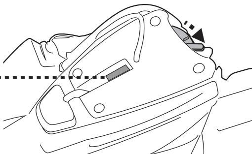
3. Slide the power switch to “ON” (while the robot is still submerged) – the indicator light will turn on and activate the motor automatically (water level covering the sensors at the top of the swivel head). Let the robot sink to the pool floor and observe its first forward and reversed movements across the pool bottom. If it runs along the pool wall instead of perpendicularly, retrieve it and redeploy it while making sure its front/back is facing the pool wall.
