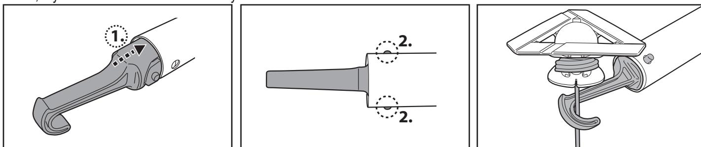
As soon as the robot reaches the water surface, locate the grip that is underneath the base and indicated with the hand symbol (see diagram below) to facilitate retrieval from the pool. Make sure to always grip the robot from this end to prevent debris from falling back into the pool during retrieval.
