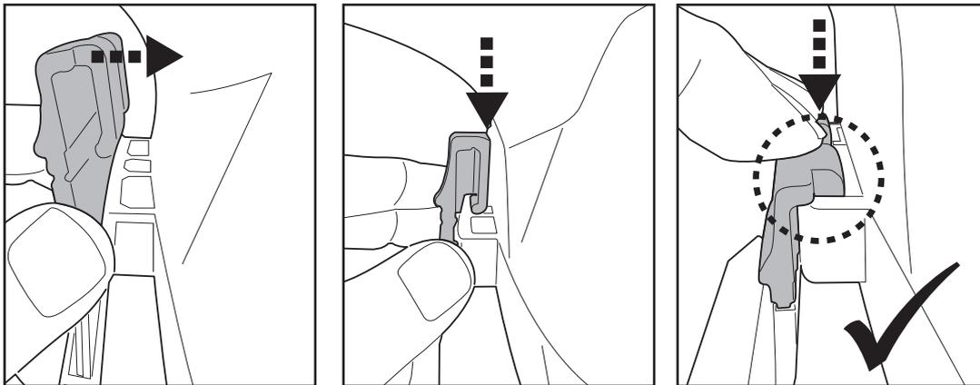
**TIPS:** Press on the two hook ends to remove the brush.
