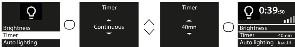
The "Auto lighting" option detects anyone in the dark and switches the light on at low brightness automatically for 30 seconds.
