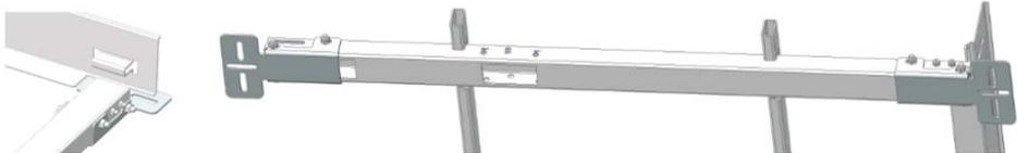
Detail of the lateral assembly, the support profiles are inserted in the base profiles:
