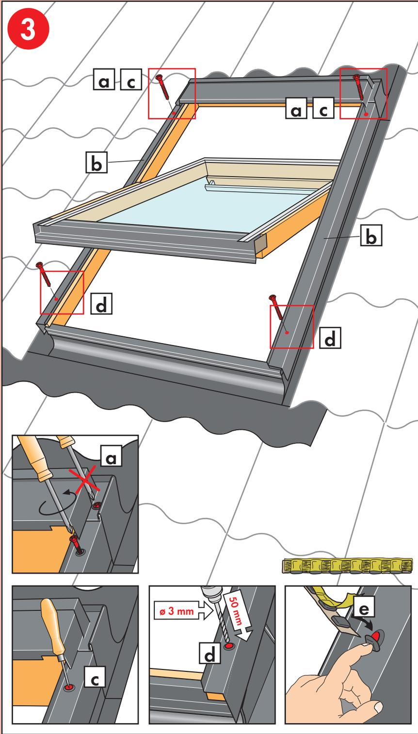
**ENGLISH:** Remove cover screws except the top cover screw [a]. The number of screws depends on the window size. Do **not** remove side frame covers [b]. If there is a mark at the top instead of a hole, make hole with bradawl [c]. Drill hole in frame, through hole in lower cover, no deeper than 50 mm using  $\varnothing$  3 mm drill [d]. Place sealant on **all** screw holes [e].
