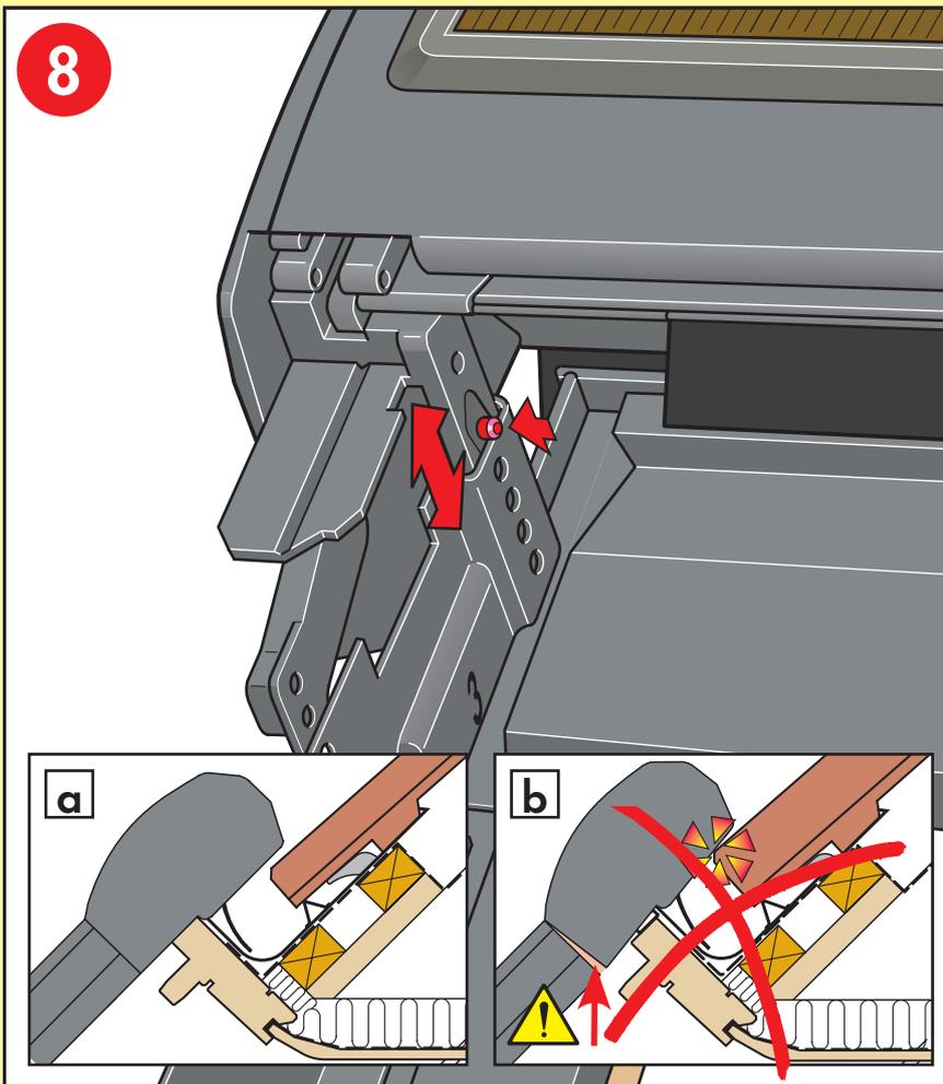
**ENGLISH:** Lower the roller shutter top casing as much as possible. Do **not** press the top casing against the roofing material **a**, **b**.
