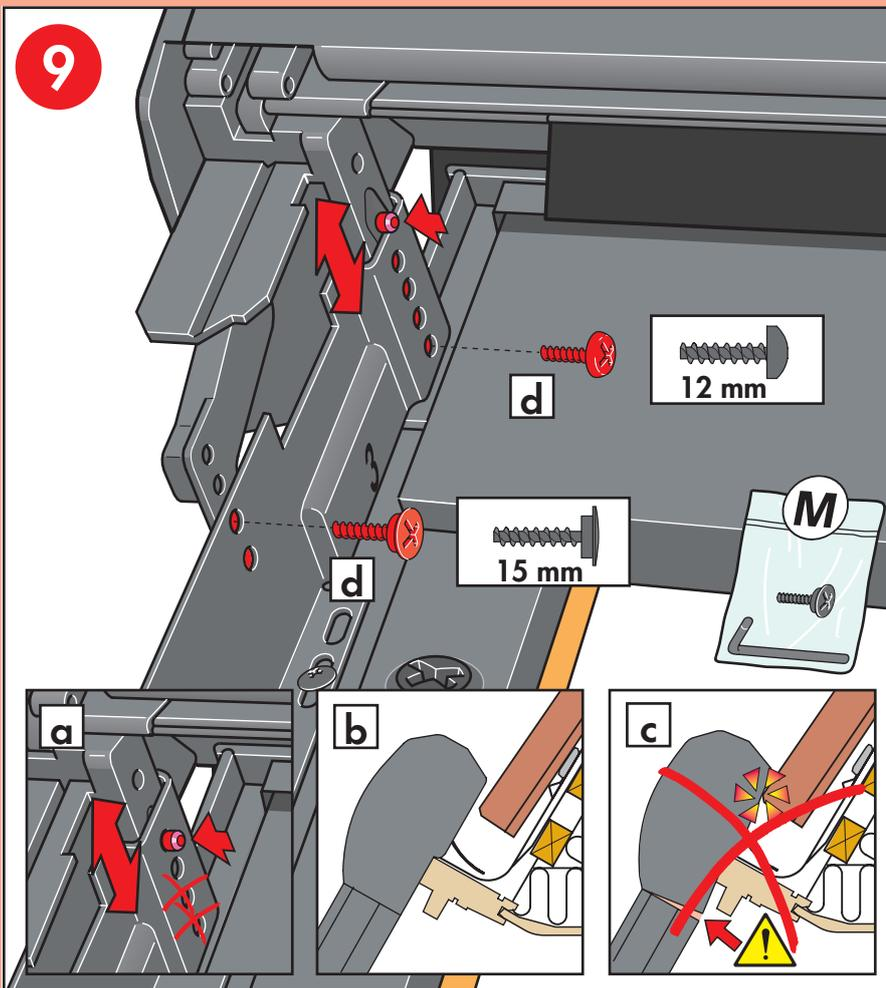
**ENGLISH:** The roller shutter top casing **must** be fitted in one of the two top holes **a**. Do **not** press the top casing against the roofing material **b**, **c**. Fit securing screws after installing the roller shutter top casing **d**.
