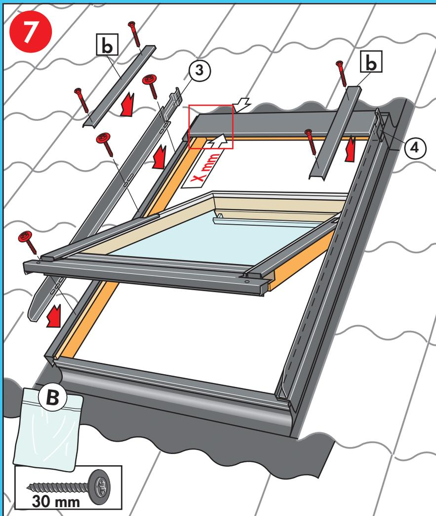
**ENGLISH:** Measure the width of the window top cover (**X mm**). Depending on this width place the roller shutter side covers as shown in the detailed drawings **A**, **B** or **C**. Fix roller shutter side covers with screws **a**. Fit window covers **b** using existing screws.
