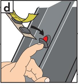
**ENGLISH:** Remove bottom cover screws. Do **not** remove side frame covers **a**. Measure the position of and drill the top hole, as shown in table **b**, **c**. Place sealant on **all** screw holes **d**.
