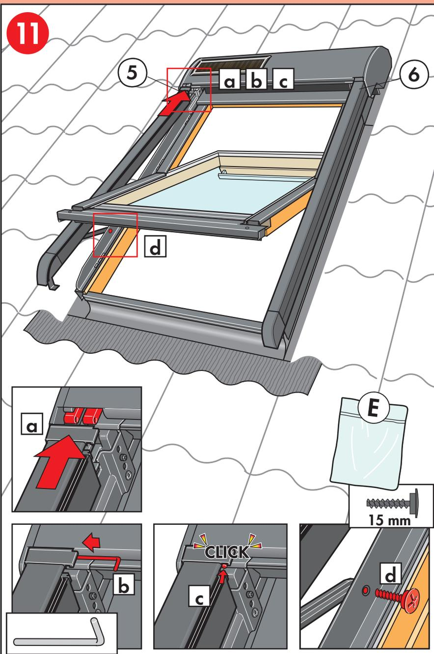
**ENGLISH:** Fit side profiles [a](#). Insert and fix pins for hinges [b](#), [c](#). Attach opening restrictors to side covers with screws [d](#).
