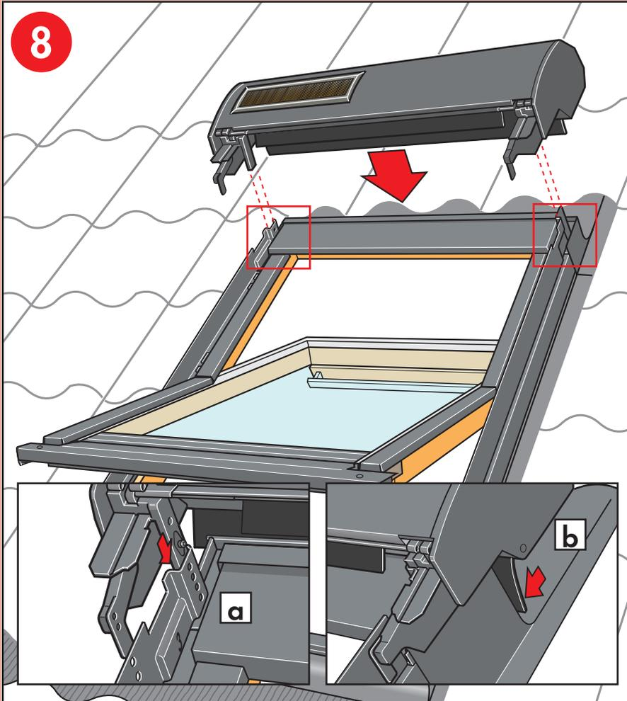
**ENGLISH:** Fit roller shutter top casing into grooves on side covers **a**. Check that rubber gasket at the back fits smoothly against outside of window **b**.
