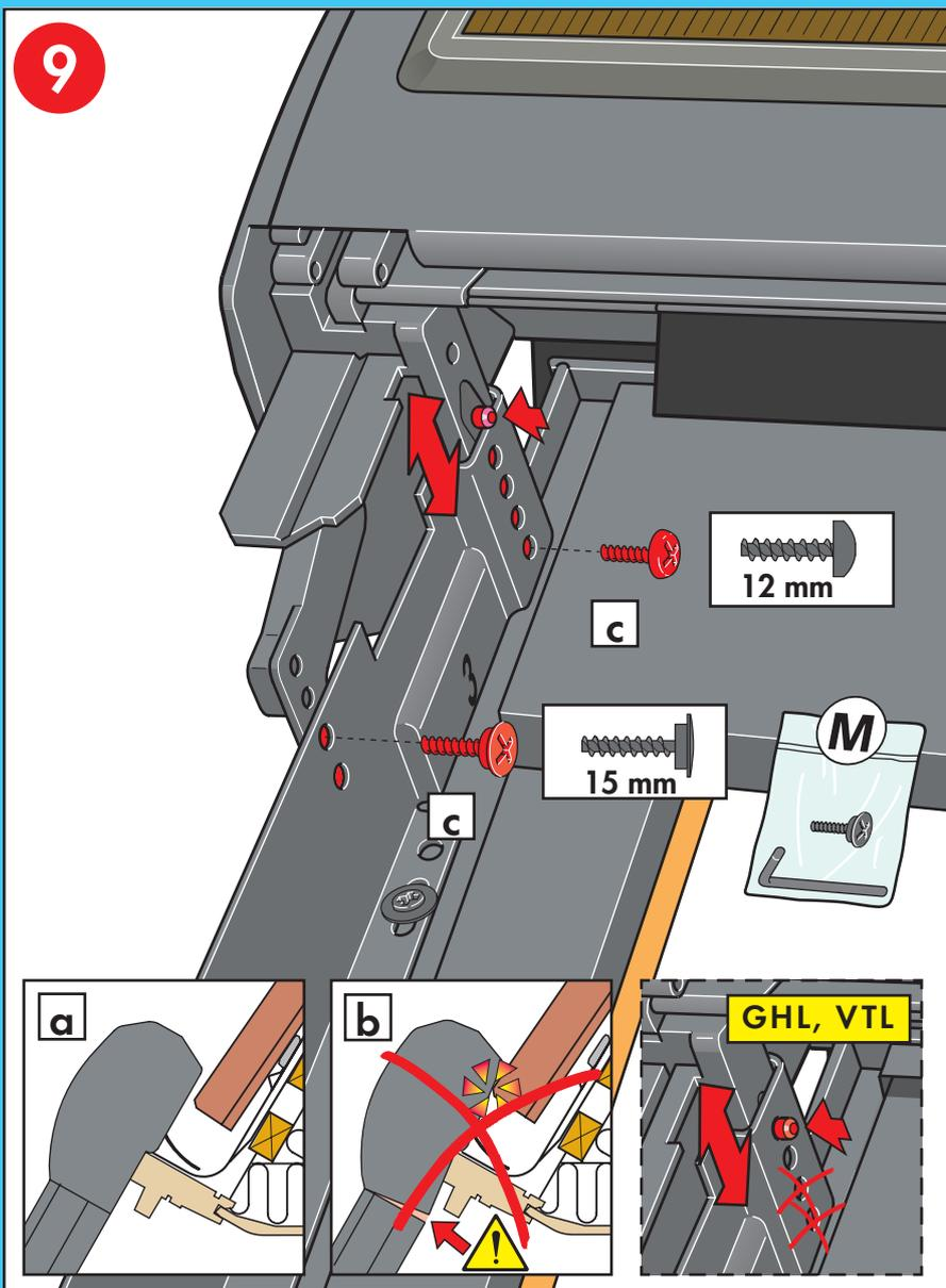
**ENGLISH:** Lower the roller shutter top casing as much as possible. Do **not** press the top casing against the roofing material **a**, **b**. Fit securing screws after installing the roller shutter top casing **c**.
