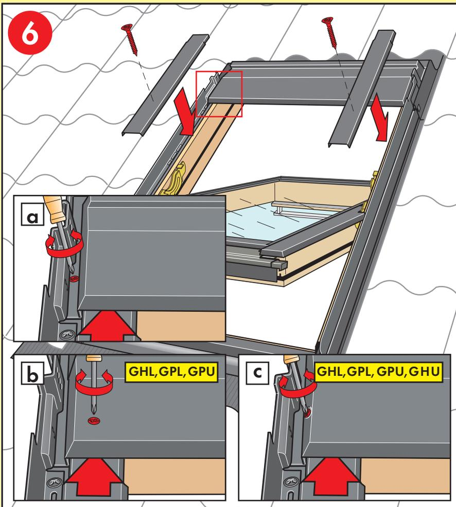
**ENGLISH:** Loosen screws in top cover [a](#), [b](#) or [c](#). Fit window covers using existing screws. Re-tighten top cover screws.
