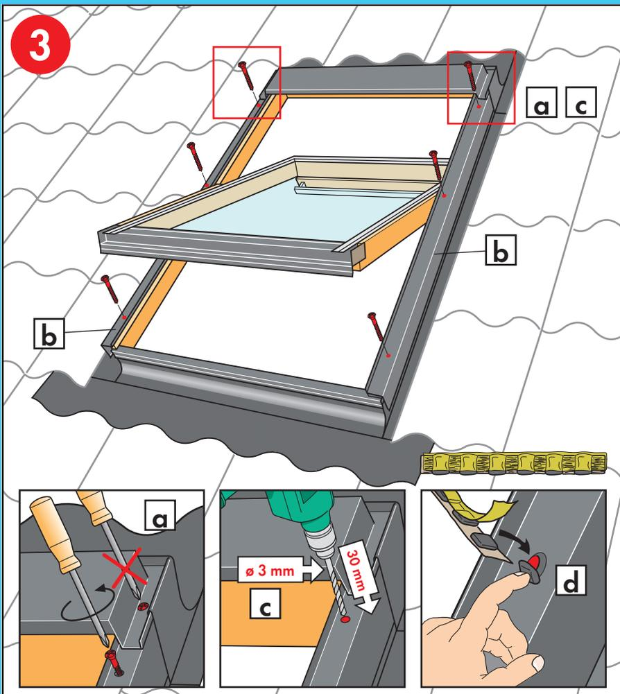
**ENGLISH:** Remove cover screws except the top cover screw [a]. The number of screws depends on the size and type of the window. Do **not** remove side frame covers [b]. If there is a mark at the top instead of a hole, drill hole at mark [c]. Place sealant on **all** screw holes [d].
