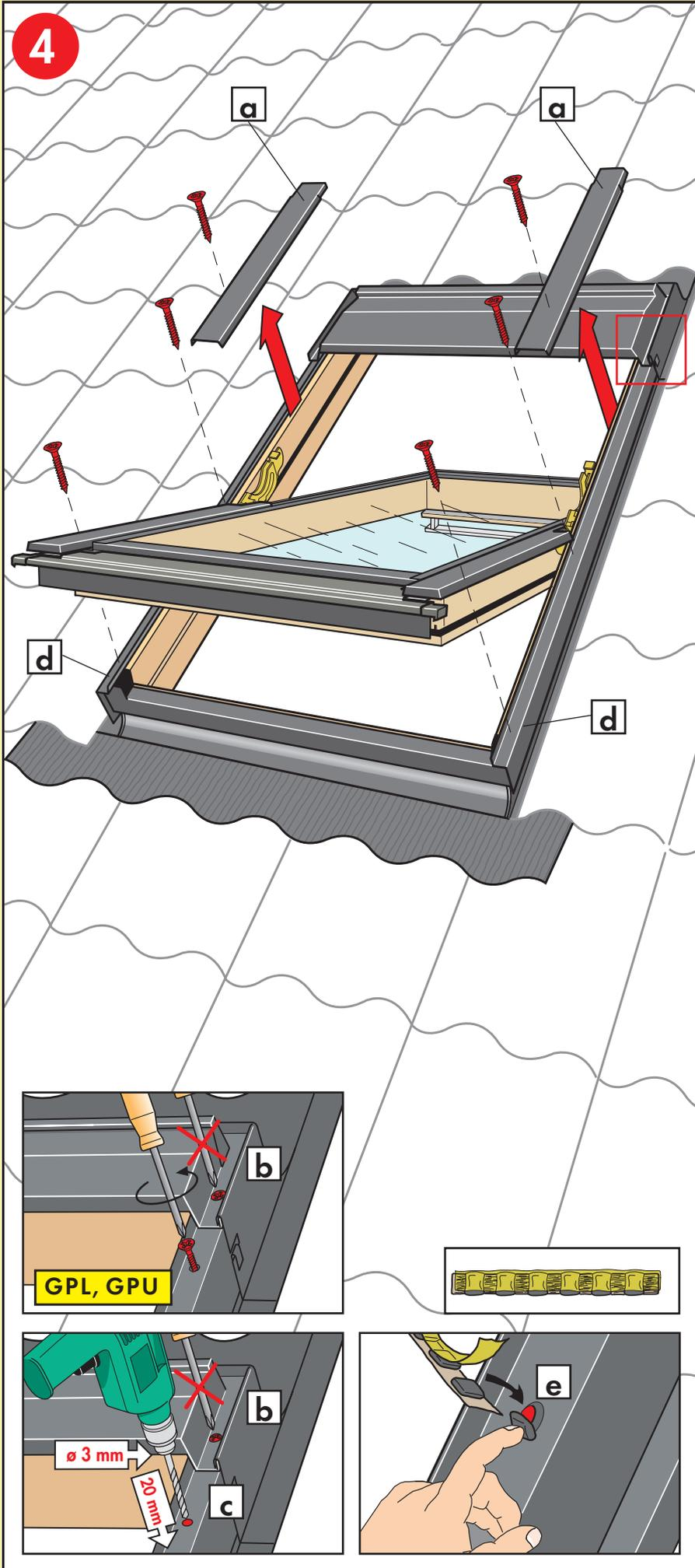
**ENGLISH:** Remove covers indicated temporarily [a]. Remove cover screws except the top cover screw [b]. If there is a mark at the top instead of a screw, drill hole through mark [c]. Do **not** remove side frame covers [d]. Place sealant on **all** screw holes [e].
