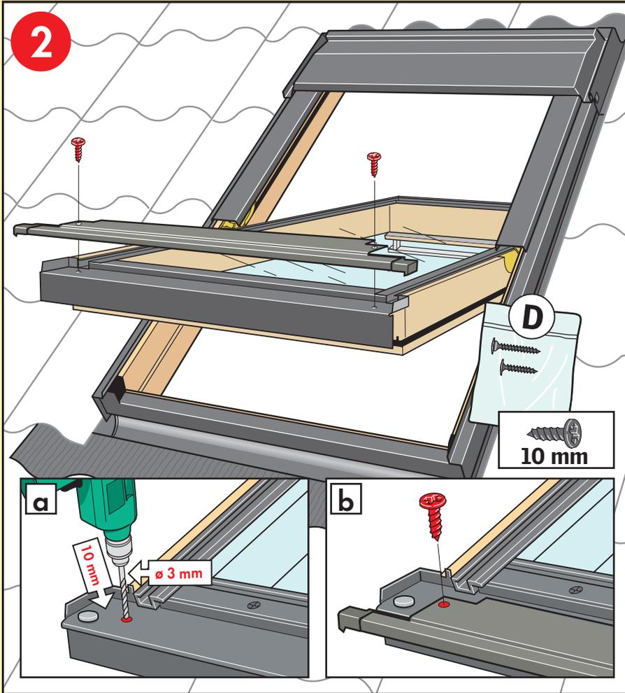
**ENGLISH:** Drill a  $\varnothing$  3 mm hole at the mark on the cover **a**. Fit bottom cover **b**.
