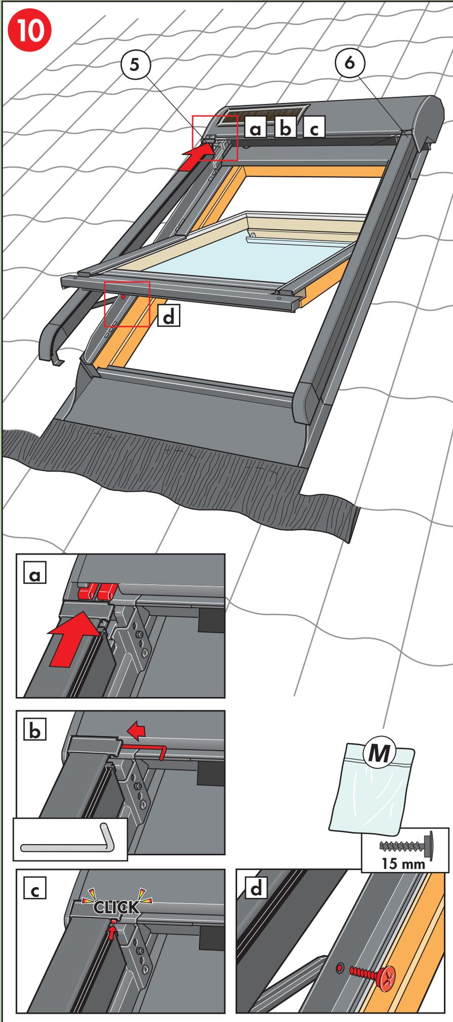
**ENGLISH:** Fit side profiles **a**. Insert and fix pins for hinges **b**, **c**. Attach opening restrictors to side covers with screws **d**.
