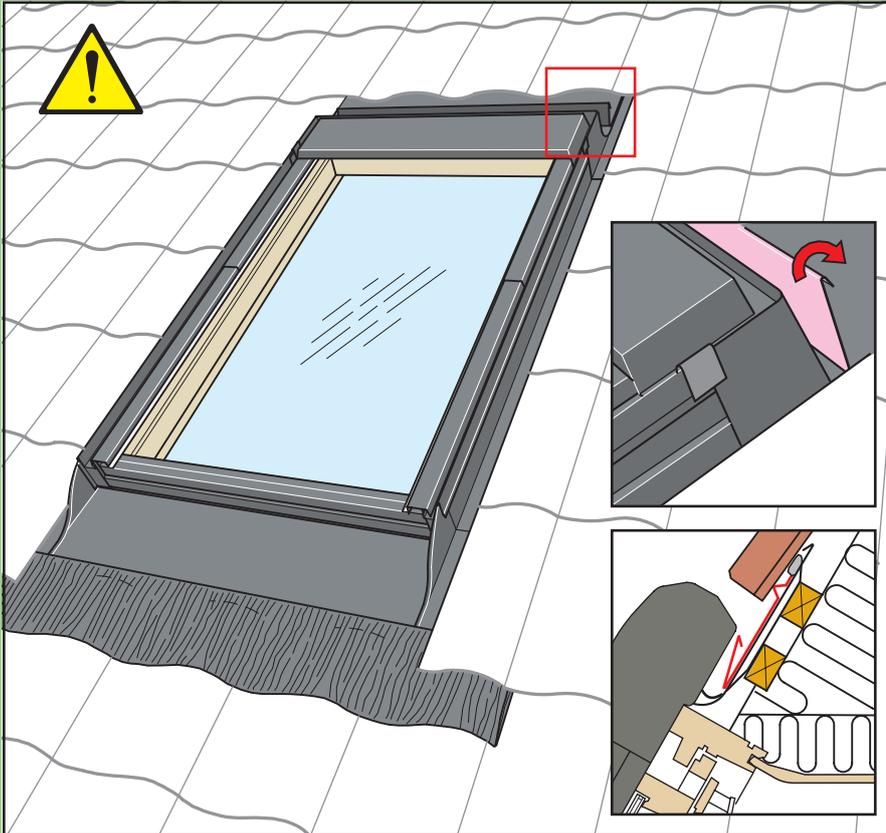
**ENGLISH:** If roller shutter is to be installed with EDJ or EDN flashing: Bend down rainwater deflector to make room for roller shutter.
