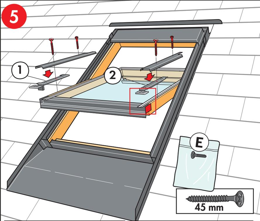
**ENGLISH:** Screw storm brackets and covers onto window sash using existing holes. Storm brackets must be positioned behind the metal flaps **a**. Use 45 mm screws supplied in the outermost holes **b** and existing screws in the innermost holes **c**.
