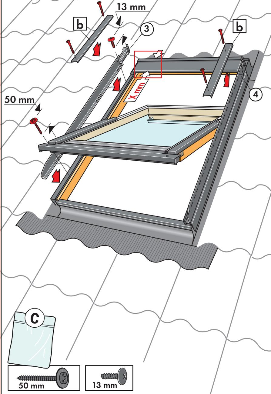
**ENGLISH:** Measure the width of the window top cover (**X mm**). Depending on this width place the roller shutter side covers as shown in the detailed drawings **A** or **B**. Fix roller shutter side covers with screws **a**. Fit window covers **b** using existing screws.
