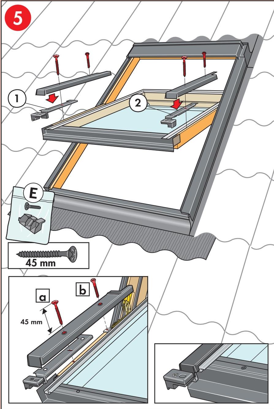
**ENGLISH:** Screw storm brackets and covers onto window sash using existing holes. Use 45 mm screws supplied in the outermost holes **a** and existing screws in the innermost holes **b**.
