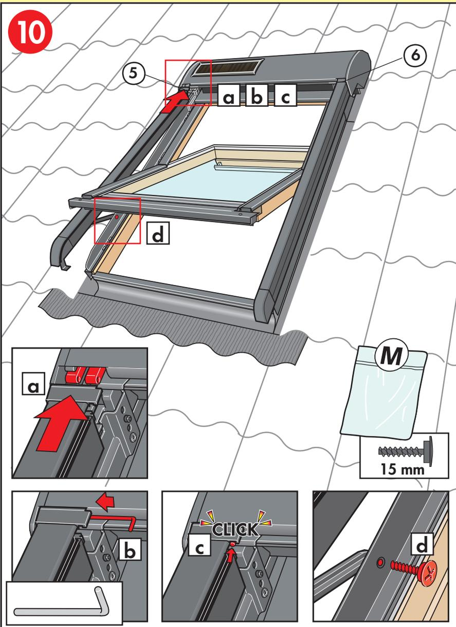
**ENGLISH:** Fit side profiles **a**. Insert and fix pins for hinges **b**, **c**. Attach opening restrictors to side covers with screws **d**. **The roller shutter is now ready for use. For important information, see pages 38-39. For operation of the roller shutter, see enclosed directions for use.**
