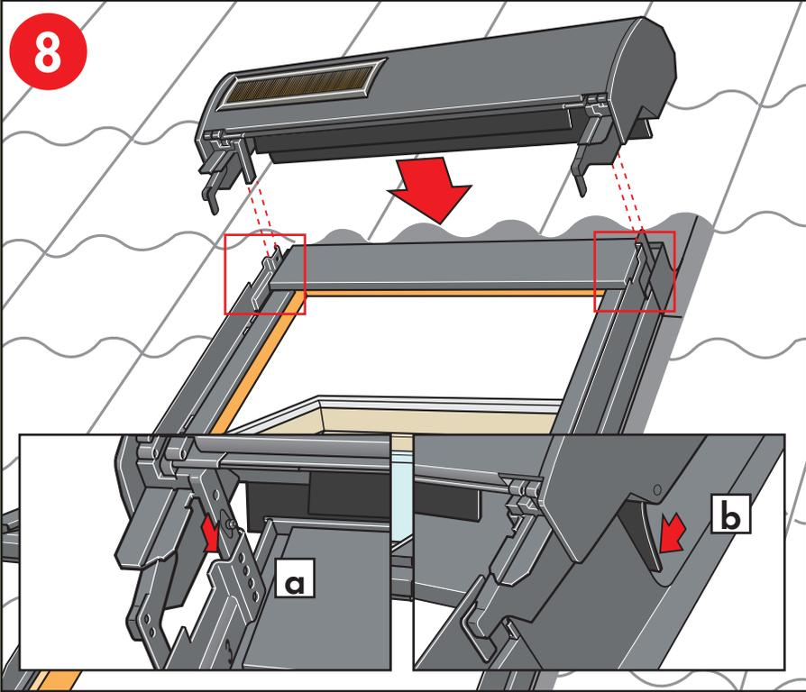
**ENGLISH:** Fit roller shutter top casing into grooves on side covers **a**. Check that rubber gasket at the back fits smoothly against outside of window **b**.
