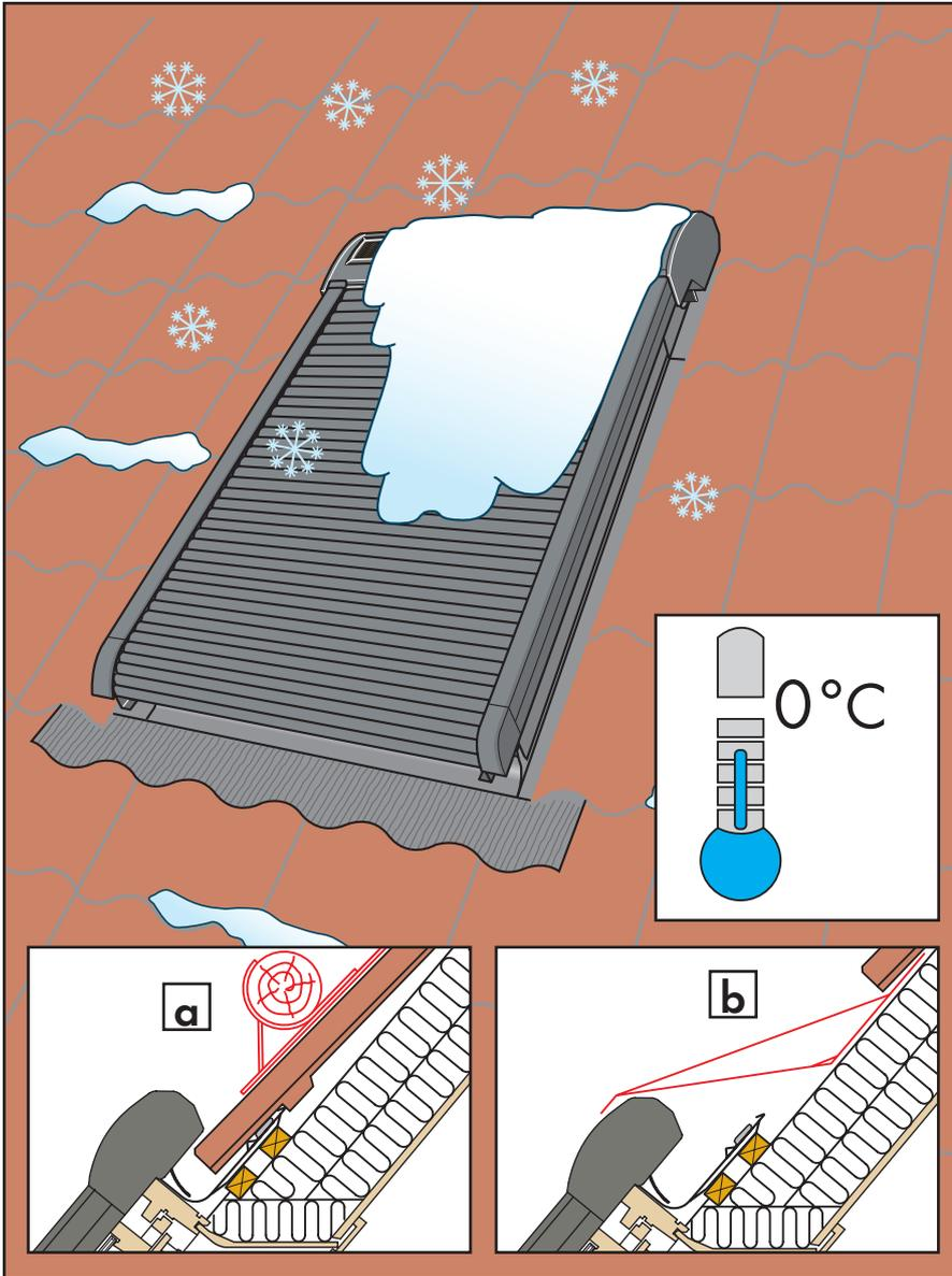
**ENGLISH:** As a precondition of avoiding any damage to the roller shutter in very cold regions and in regions with heavy snowfall, either a snow stop or wedge must be installed above the roller shutter [a](#), [b](#). The roller shutter is protected against overload, and will stop automatically if it is blocked.
