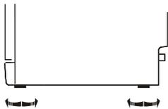
Once the appliance is positioned for levelling, the height of the dishwasher may be altered by adjusting the screwing level of the feet. In any case, the appliance should not be inclined more than 2°.
