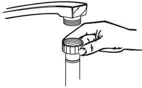
Connect the cold water supply hose to a threaded 3/4(inch) connector and make sure that it is fastened tightly in place.
