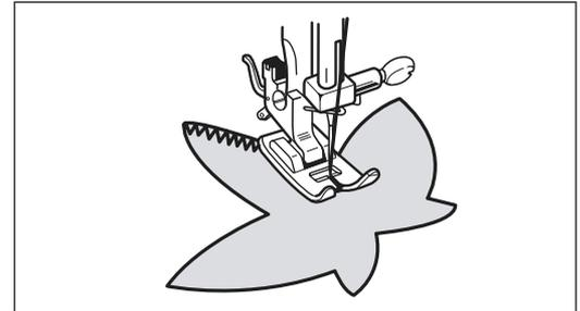
To change direction at corners, or to sew very small circles, stop machine, positioning needle just away from edge of cut-out, lift presser foot and turn material. Lower presser foot and continue sewing.
