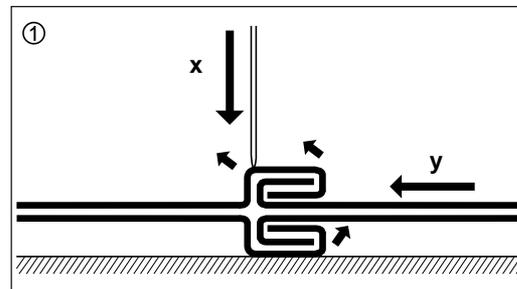
Improper setting causes deflection and possible breaking of the needle.
