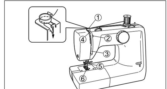
Lead thread through either side of tension disc ②.
