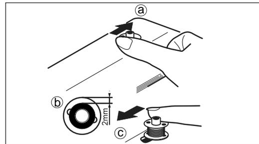
Note: Watch the bobbin carefully to wind the correct volume of thread.
