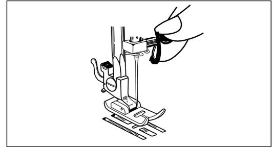
With the flat side away from you, insert a new needle into groove of needle bar.
