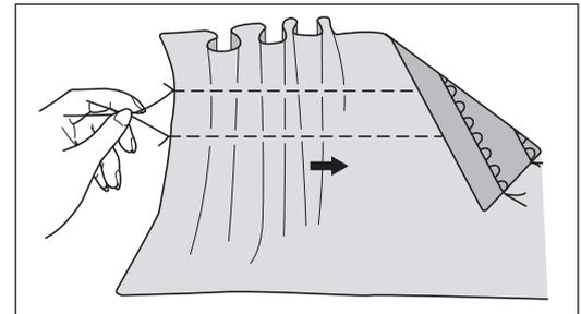
Sew smocking stitches on gathered part between two straight lines of stitches. Take out the threads of the straight stitching after you finish sewing.
