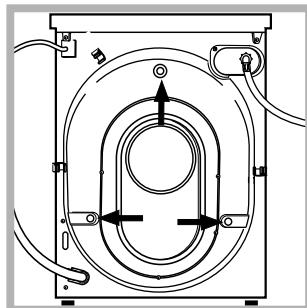
3. Remove the 3 protective screws and the rubber washer with the respective spacer, situated on the rear of the appliance (see figure).
