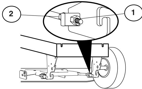
**(GB)** To obtain the best cutting results, the mower blades should be adjusted so the front tip (B) is approximately 1/8" to 1/2" lower than the rear tip (A) when the mower is in its highest position.
