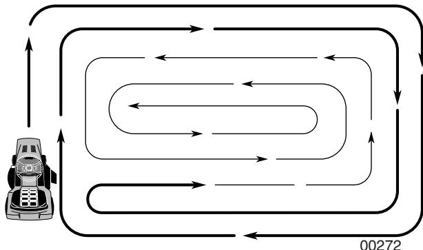
**(GB)** Use the left side of the machine to cut close to trees, bushes and paths, etc. The blade cuts about 15 mm inside the edge of the cover.
