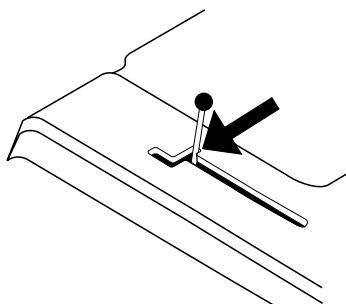
GB Press down the clutch/brake pedal completely and hold down. Make sure that the motion control lever is in neutral "N".
