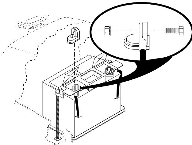
**(GB)** **NOTE:** If battery is put into service after month and year indicated on label, charge battery for minimum of one hour at 6-10 amps.
