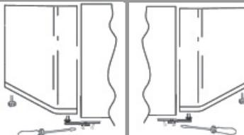
Remove the caps (A) and (B), loosen the screws and partially remove the panel.
