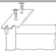
Remove the plug on the left-hand side and insert it on the right hand-side of the door.
