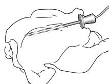
For poultry, the probe should be inserted sideways, in the middle of the breast, taking care to ensure the tip does not end up in a hollow part. In the case of meat with very irregular thickness, check it is cooked properly before removing it from the oven. Connect the end of the probe in the hole located on the right wall of the oven cavity.
