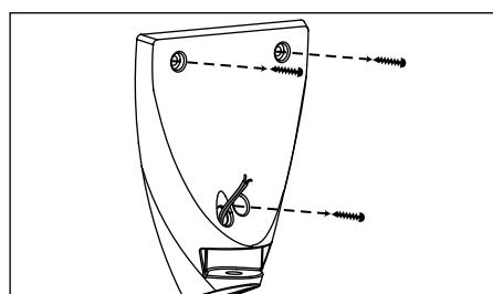
4. Use the base as a template to mark the position of the three fixing screws on the wall. The three fixing holes should be drilled with a 6mm masonry bit and the plastic wall plugs firmly inserted until they are flush with the wall surface.
