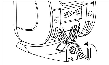
2. Use the hexagonal key supplied in the base of the Sib to unscrew the bolt that holds the base to the support bracket
