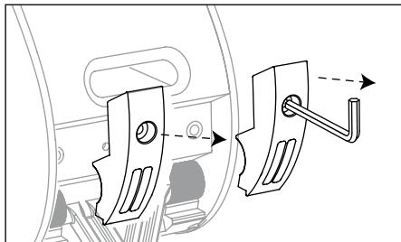
6. Remove the silver support piece, turn it 180°, and reposition the support so that it will fit horizontally with the wall mounted base.
