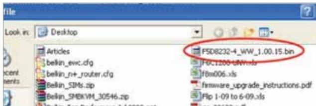
8. Select the firmware file by left-clicking on it and then click the “Open” button in the lower-right corner of the window. This will take you back into the Router’s interface.
