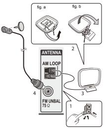
1 Push open the tabs, then insert one wire fully into each terminal, then release the tabs to secure the AM antenna wires.
