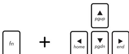
Press <Fn> and the arrow keys to scroll up and down or scroll to the start and end of a document or web page.
