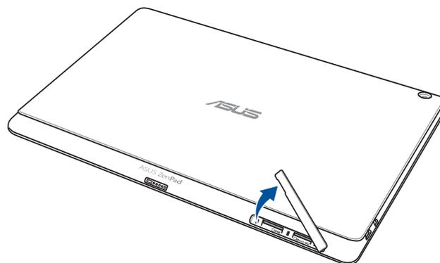
2. Align and insert a micro SIM card into the micro SIM card slot.
