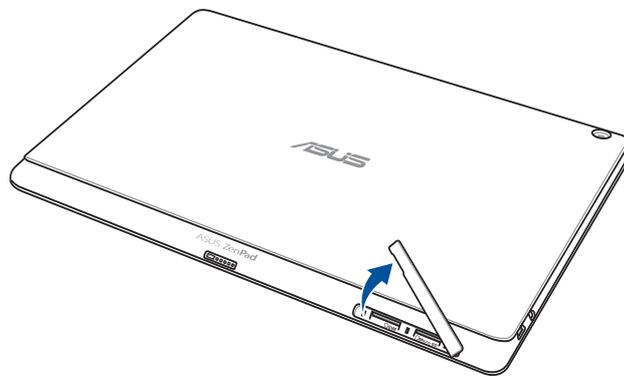
2. Press the micro SIM card to eject, then pull it out.
