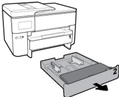
2. Check the gap in the printer where the input tray was. Reach into the gap and remove the jammed paper.
