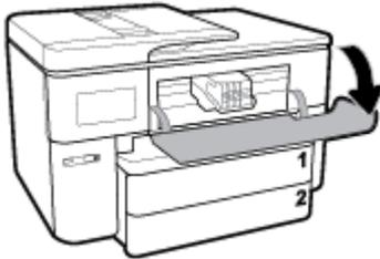
2. If the print carriage is not obstructed, move the print carriage to the far right of the printer and remove the jammed paper.
