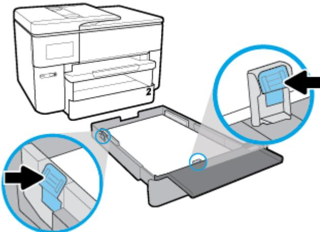
7. Check the input tray area inside the printer. If there is paper, remove the paper.
