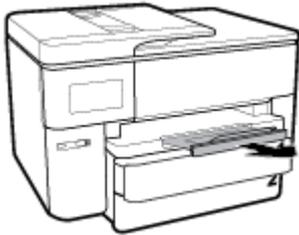
Pull out the output tray extension to the B size marking.
