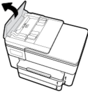
This provides easy access to the rollers (1) and separator pad (2).
