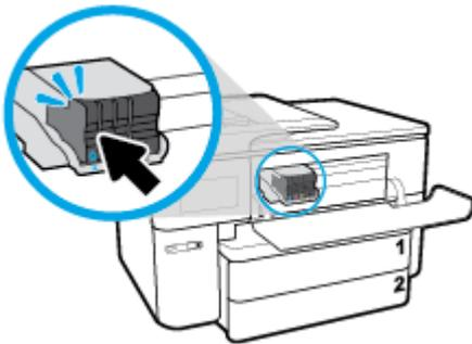
Make sure that the color-coded letter on the cartridge matches that on the slot.
