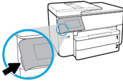
**NOTE:** Return the control panel to its original position by pushing down the left side until it back into place.
