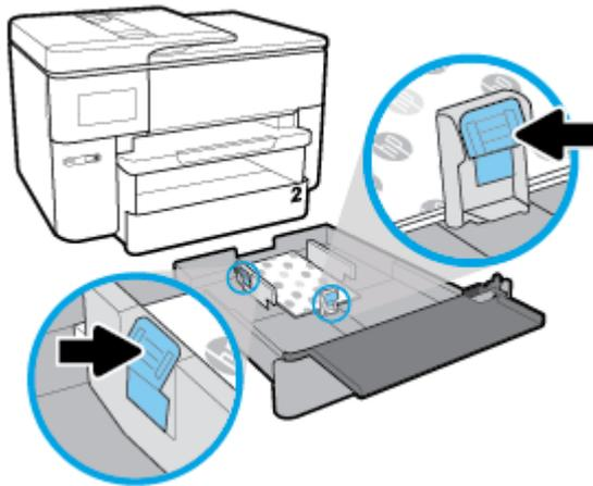
6. Check the input tray area inside the printer. If there is paper, remove the paper.
