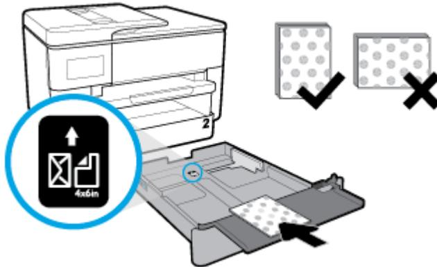
Make sure the stack of card or photo is aligned with the appropriate paper size lines on the front of the tray. Also, make sure the stack of card or photo does not exceed the stack height marking on the right edge of the tray.
