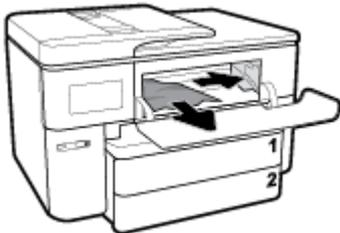
If necessary, move the carriage to the far left of the printer, and remove any jammed or torn pieces of paper.
