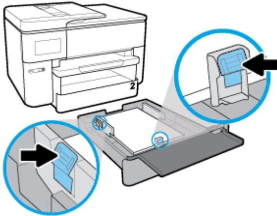
5. Check the input tray area inside the printer. If there is paper, remove the paper.
