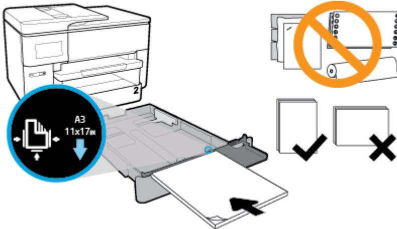
Make sure the stack of paper is aligned with the appropriate paper size lines on the front of the tray. Also, make sure the stack of paper does not exceed the stack height marking on the right edge of the tray.
