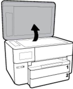
2. Load your original print-side down and align it with the marking on the rear left corner of the glass.
