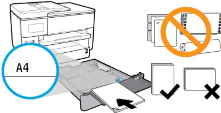
Make sure the stack of paper is aligned with the appropriate paper size lines on the front of the tray. Also, make sure the stack of paper does not exceed the stack height marking on the right edge of the tray.
