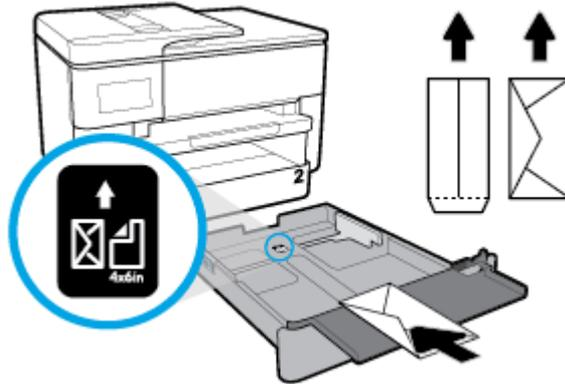
Make sure the stack of envelope is aligned with the appropriate paper size lines on the front of the tray. Also, make sure the stack of envelope does not exceed the stack height marking on the right edge of the tray.
