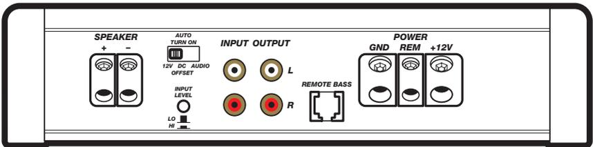
**Automatic Turn-On Selection:** The IX series offers three different automatic turn-on modes that can be selected on the end panel; +12V, DC Offset, and Audio. Using either the DC Offset or Audio mode causes the REM terminal to have +12V out for turning on additional amplifiers.
