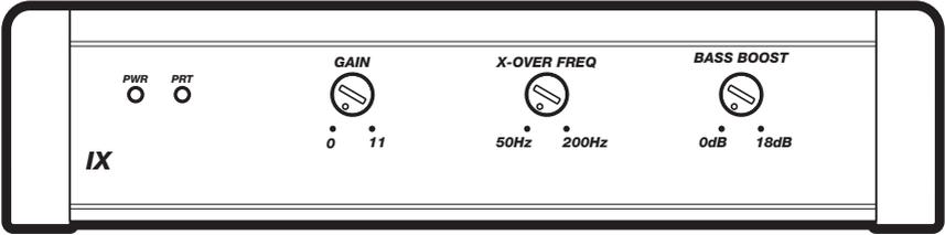
**Input Gain Control:** The input gain control is not a volume control. It matches the output of the source unit to the input level of the amplifier. Turn the source unit up to about 3/4 volume (if the source unit goes to 30, turn it to 25). Next, slowly turn (clockwise) the gain on the amplifier up until you can hear audible distortion, then turn it down a little.
