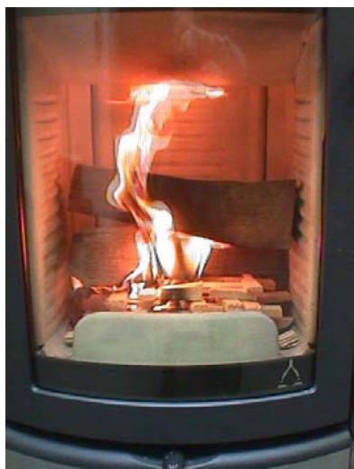
Figure 5: Close the Primary Air
