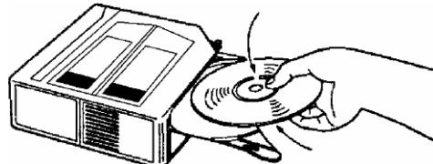
3. Push the tray back into the magazine. Load additional discs into the remaining nine trays in a similar manner.
