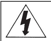
The lightning flash with arrowhead, within an equilateral triangle, intended to alert the user of the presence of uninsulated „dangerous voltage“ within the product's enclosure; that may be of sufficient magnitude to constitute a risk of electric shock to persons!
