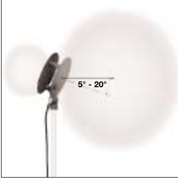
Fig. 4: Hypercardioid polar pattern.
