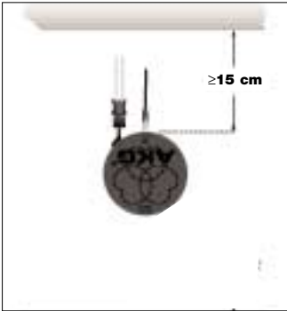
Fig. 7: Minimum distance from the ceiling.
