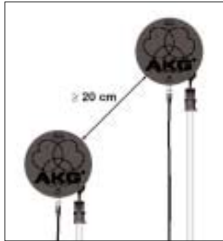
Fig. 8: Minimum distance between two antennas.
