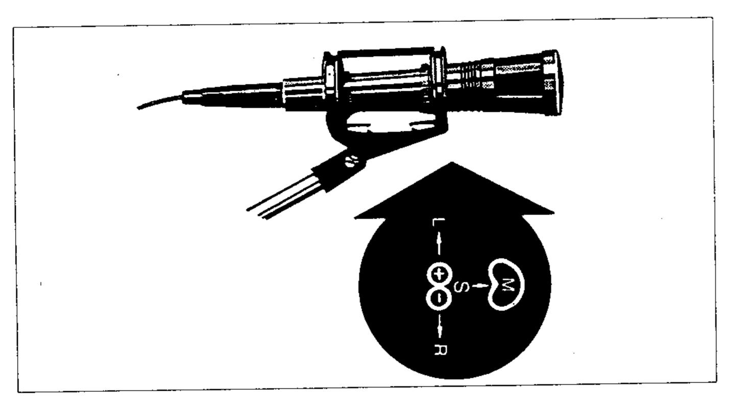
For correct left/right orientation, be sure to mount the microphone in such a way that the symbols shown always face up.
