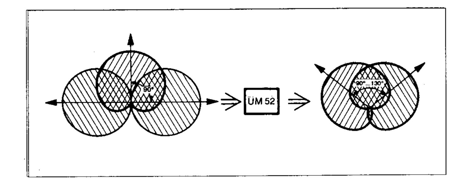
For stereo playback, M-S-signals must obviously be processed in some way to obtain Left-Right information. Mathematics tell us that the addition M+S provides the left channel signal, while the right channel signal is derived from the subtraction M-S. In practice, these "calculations" can be done either by connecting the M and S microphones to four mixer inputs as shown in the next figure or to the matrix box UM 52.
