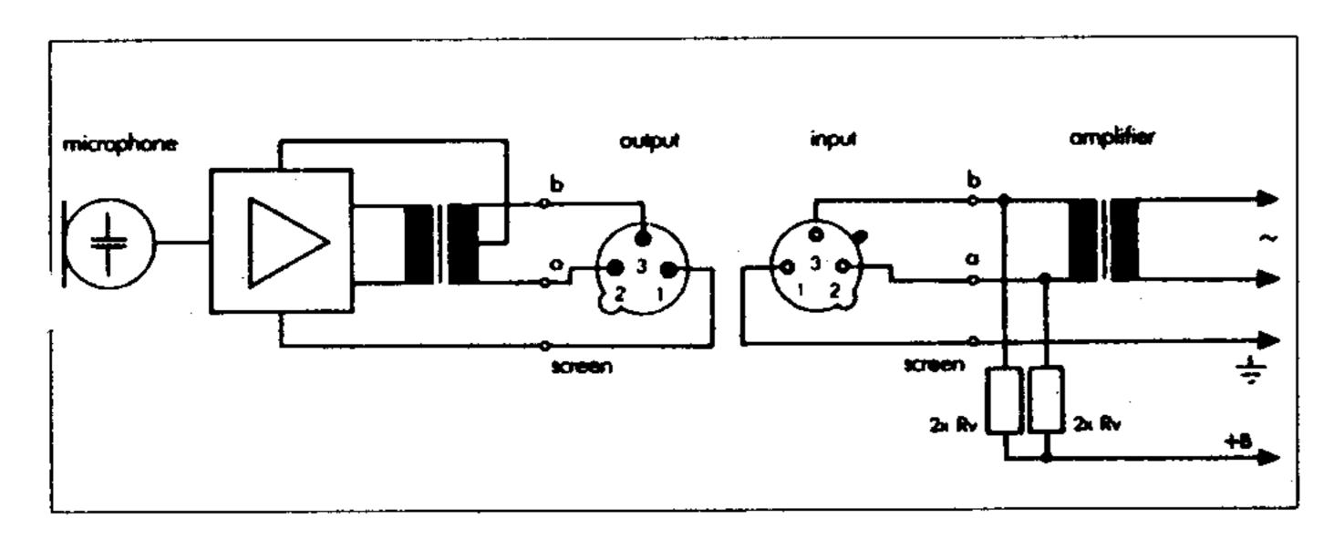
The resistors 2x Rv must have a tolerance not exceeding 0.5% in order to satisfy the symmetry requirement.
