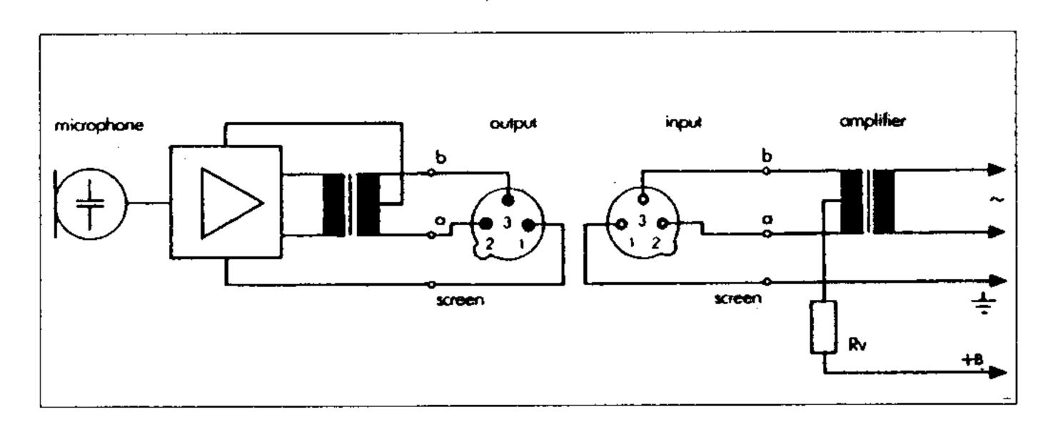
Input circuitry incorporating transformer without center tap (ungrounded)
