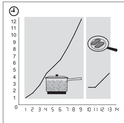
You can get a necessary heat setting in a shorter time if you activate the Automatic Heat Up function. This function sets the highest heat setting for some time (see the graphic), and then decreases to the necessary heat setting.
