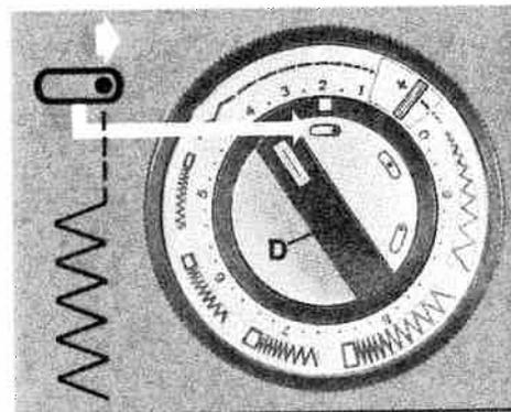
**3** Right needle position: the needle enters the needle hole on the right.
