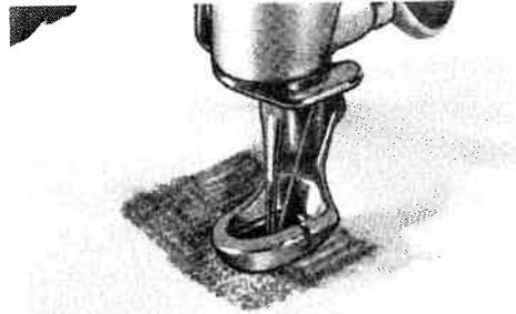
Hold the material flat with both hands. Stitch back and forth across the hole lengthwise, with the machine running at high speed. Be sure the stitches are closely spaced. Then turn the fabric at right angles and sew back and forth over the preceding work with short stitches. This anchors the threads in the unworn area around the hole.
