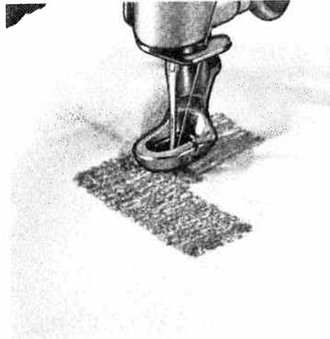
After you have finished darning, swing the reverse-feed control back to its regular sewing position.
