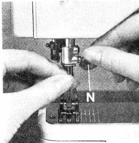
Changing the sewing foot is just as simple. The accessory box of your machine contains several special sewing feet (hemmer foot, buttonhole foot, etc.) which are used for various sewing operations. Which sewing foot to use for a specific sewing job is discussed on page 23 and the following pages.
