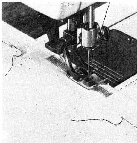
Rip open the section of the hem opposite the damaged area. Take a piece of suitable material in the right size, fold it in half and press. Then insert this piece in the hem so that its folded edge is in line with the folded edge of the hem.
