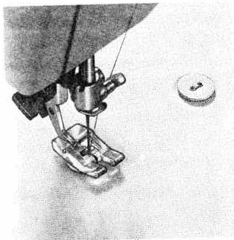
Place the material and the button under the sewing foot and align them so that the needle will enter the right hole in the button. Check the correct position of the button by letting the needle stitch through the hole. Sew one or two tying stitches, then raise the needle again.
