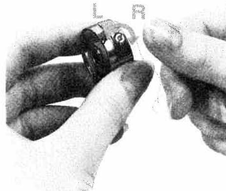
The **lower tension** is regulated by turning the small knurled screw on the bobbin case. Turn this screw to the right (with your thumb rather than your finger nail) for a tighter tension, or to the left for a looser tension. Right (R) and left (L) are indicated by arrows.
