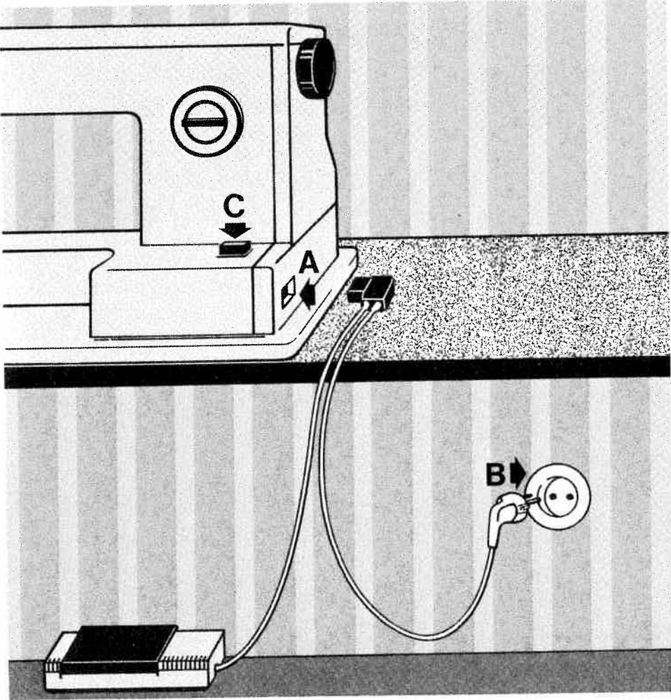
only a few simple steps are necessary. Just plug in the machine, wind the bobbin and thread the needle. Push the master plug into socket **A** in the machine base, and plug **B** into the wall socket.
