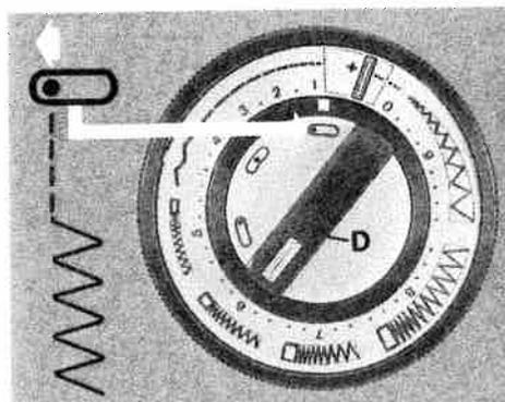
**2** Left needle position: the needle enters the needle hole on the left.
