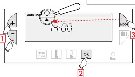
**1** Set the time using the **+/**- buttons (the numbers run off more quickly when the button is pressed continuously).
