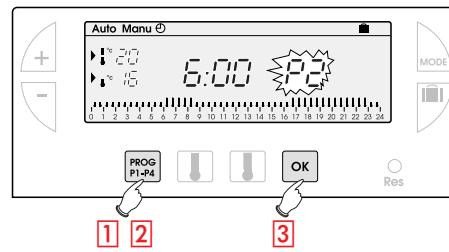
**1** Press the **PROG P1-P4** button to go into programming mode.
