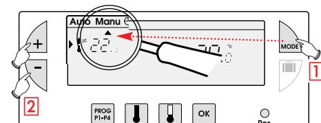
**1** Press the **MODE** button to position the pointer **▲** under **Manu**.
