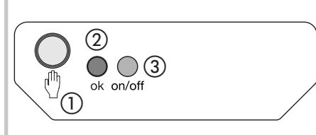
In order to associate the transmitter with the receiver:
