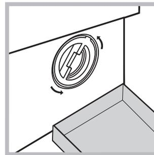
2. position a container so that it will collect the water which flows out (approximately 1.5 l) (see figure);
