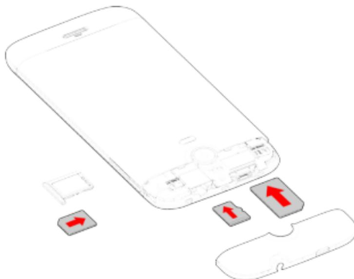
The holder on the right in the same slot is for installing a MicroSD memory card (up to 32GB). Insert the SD card gently as shown in the diagram.
