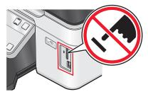
**Warning—Potential Damage:** Do not touch any cables, any network adapter, any connector, the memory device, or the printer in the areas shown while actively printing, reading, or writing from the memory card. A loss of data can occur.
