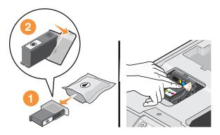
**Note:** Install the ink cartridges immediately after removing the protective cap to avoid exposing the ink to air.
