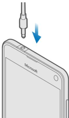
Do not connect to products that create an output signal, as this may damage the device. Do not connect any voltage source to the audio connector. If you connect an external device or headset, other than those approved for use with this device, to the audio connector, pay special attention to volume levels.
