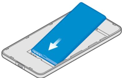
7. Press the top edge of the back cover against the top edge of your phone, and snap the cover into place.
