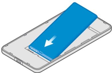
7. Press the top edge of the back cover against the top edge of your phone, and snap the cover into place. Don't press the keys while attaching the cover.
