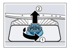
Pull down the micro filter to remove.
