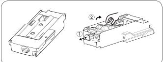
4. After cleaning the tray, put it back in, then firmly push in the icemaker, close the freezer drawer, and switch on the icemaker function via the display panel.
