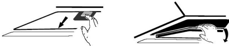
Plug the activated carbon filter into the unit and turn it in clockwise direction. Repeat the same on the other side.
