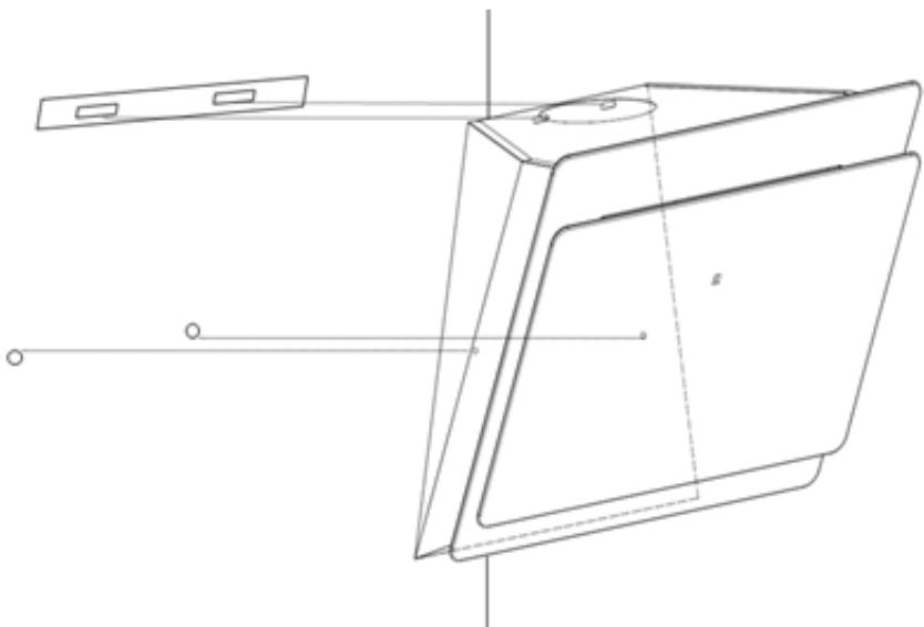
4. Leave up the cooker hood and hang onto the wall bracket hook.
