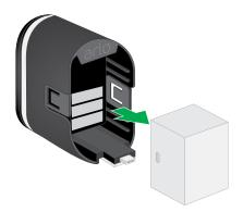
4. Align the battery and insert it into the battery compartment. The battery only inserts one way.
