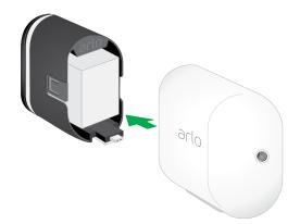
3. Remove the battery by pulling on it until it slides out of the camera.
