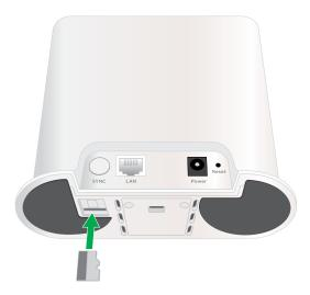
2. Press the edge of the microSD card until it's completely seated in the slot.
