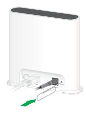
When the SmartHub reset completes, the LEDs on the front of the SmartHub blink amber. When the LEDs stop blinking amber, your SmartHub reboots. The SmartHub is removed from your Arlo account.
