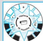
The replacement symbol will remind you during the next 7 shaves to replace the foil and cutter cassette. Then the shaver will automatically reset the display.
