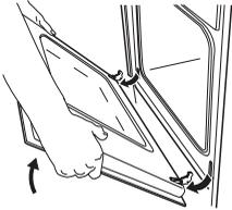
Close the oven door to the first opening position (halfway). Then pull forward and remove the door from its seat.
