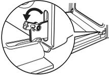
Lift and turn the levers on the two hinges.
