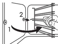
Pull the rear end of the shelf support away from the side wall and remove it.
