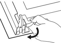
Release the locking system to remove the glass panels.
