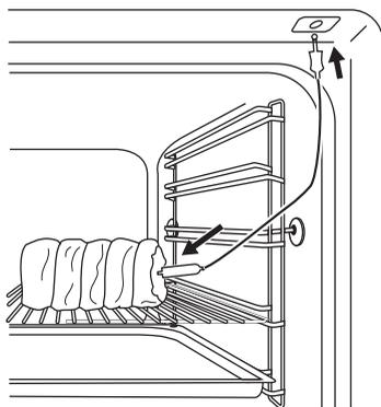
1. Put the tip of the core temperature sensor (with
