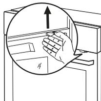
To open the oven door with the child lock installed, pull the child lock handle up as shown in the picture. Close the oven door without pulling the child lock.
