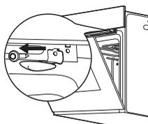
To remove the child lock, open the oven door and remove the child lock with the torx key. The torx key is in the oven fitting bag.
