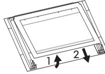
Carefully lift (step 1) and remove (step 2) the glass panels one by one. Start from the top panel.
