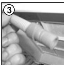
4. Attach the black hose from the kit, (using the connector and pipe clips supplied), to the hose removed from the bridge connection.
