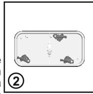
3. Gently remove the filter frame and clean any dust or fluff with a cloth from the filter. Do not use water to clean the filter.
