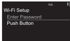
3. If you select "Enter Password", enter the password of the access point. For details on how to enter text, refer to "Entering text" (➔P36).
