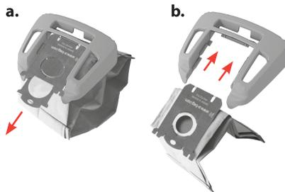
5. a) Pull the cardboard to remove the s-bag® from the insert. This automatically seals the s-bag® and prevents dust leaking out.
