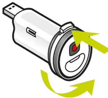
2. When you see a dot and arrow to the left of the release lever the Batt-Stick can be inserted as described above.
