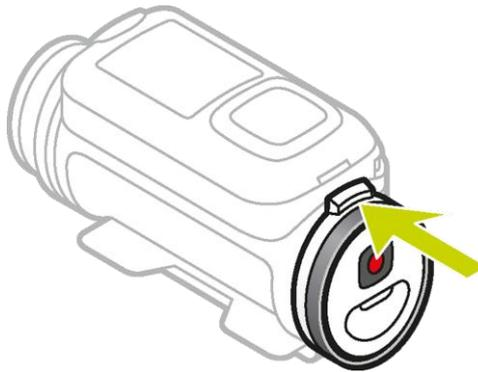
2. While holding the lever turn the cap anti-clockwise until you see two dots aligned.
