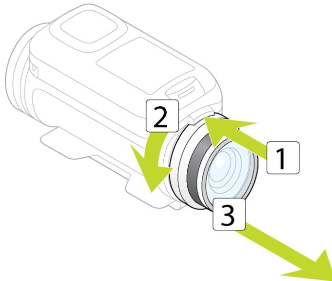
To install a lens cover, put the lens cover on the TomTom Bandit lens and turn it clockwise until it locks.
