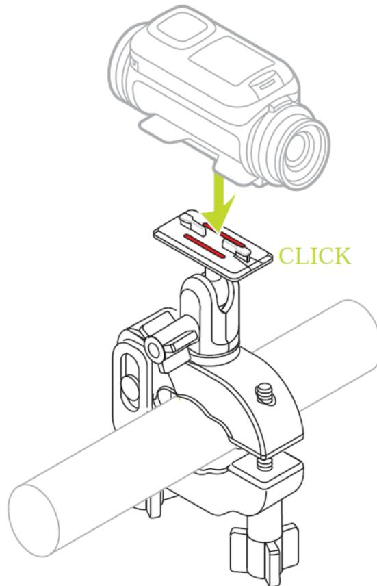
Install the bike mount only on a clean and dry surface. Wax, oil, dirt and moisture will reduce grip, causing the mount to move.
