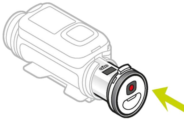
2. Make sure the two dots align and are close together.
