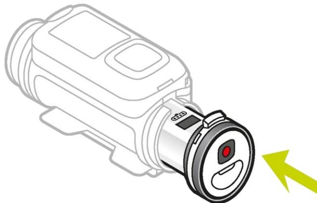
5. Make sure the two dots align and are close together.
