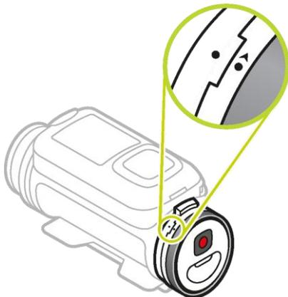
3. Turn the cap clockwise to lock the Batt-Stick into the camera.
