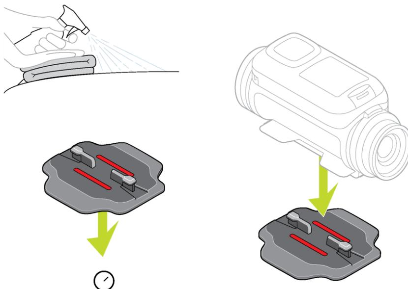
3. Make sure the mount is aligned in the correctly direction then, in dry, room-temperature conditions, attach the mount. Push the mount firmly down on to the surface.
