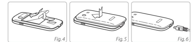
**Fig. 4:** The battery contacts have to touch the gold coloured contacts of the mobile phone.
