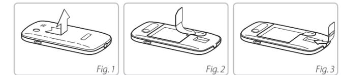
**Fig. 1:** Remove the battery cover
