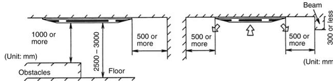
\* If the height from the floor to ceiling exceeds three meters, air flow distribution deteriorates and the effect is decreased.
