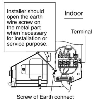
Installer should open the earth wire screw on the metal part when necessary for installation or service purpose.
