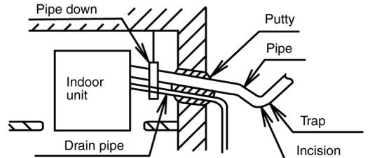
\* Put the incision at the trap part of the heat insulator (for water drain)
