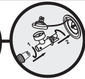
Ensure that the inner spring valve is not depressed. ( If depressed, press the spring valve and turn counter clockwise ) Attach the pressure gauge onto the hose of SPA pump, inflate the spa to 0.008MPa ( 1.2PSI )
