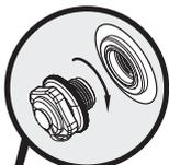
Screw the screw-valve onto the air intake valve marked with No. 1 on the spa.
