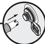
Open the top cover of the screw-valve, insert the inflation hose and inflate. Once inflation is finished, fasten the top cover of the screw-valve.
