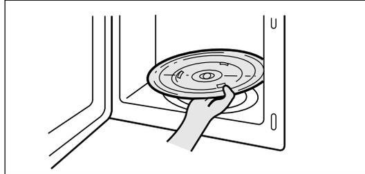
7. The roller guide and oven cavity floor should be cleaned regularly to avoid excessive noise. Simply wipe the bottom surface of the oven with mild detergent water or window cleaner and dry. The roller guide may be washed in mild sudsy water.
