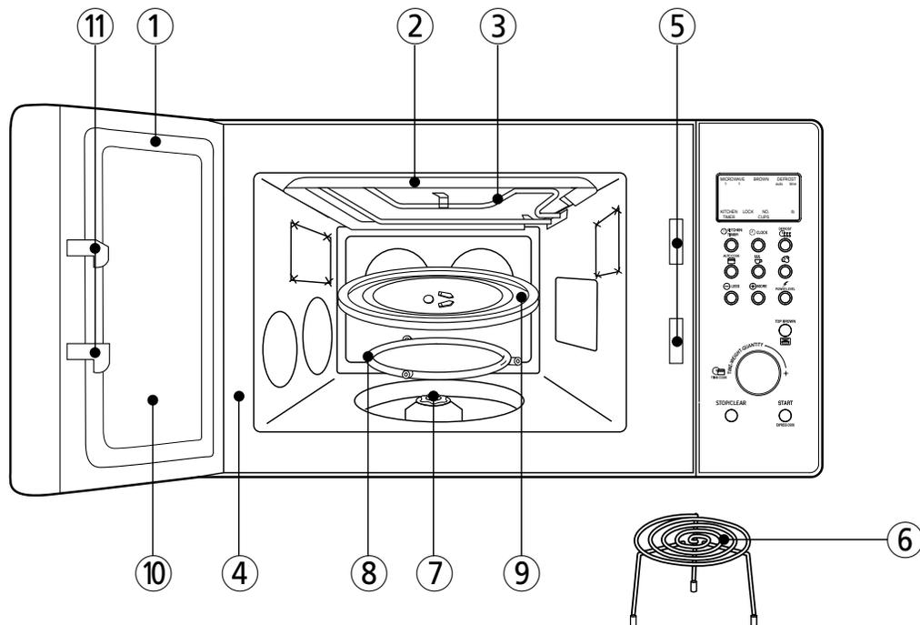
**1. Door seal** - Door seal maintains the microwave energy within the oven cavity and prevents microwave leakage.
