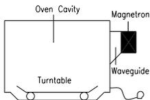
In a microwave oven, electricity is converted into microwave by the **MAGNETRON**.
