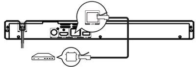
1. Connect the network cable from the LAN jack on the product to the LAN jack on the network system.
