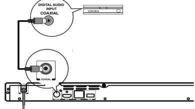
1. Connect a coaxial cable from the COAXIAL jack on this product to the COAXIAL jack on the device.
