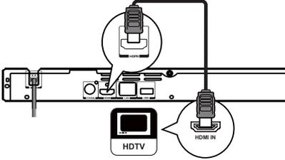
1. Connect a HDMI cable from the HDMI output jack on this product to the HDMI input jack on the TV.
